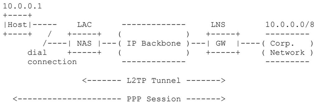
Figure 6.1: Compulsory Tunneling Example
